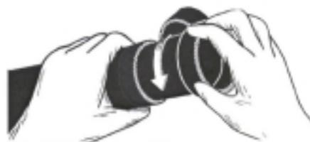
Remove the threaded cap of the cleanout tee. Place one unopened bag of rodent bait pellets into the center and replace the cap. It is not necessary to open the bag. Let the rats chew on the bag to access the bait.
